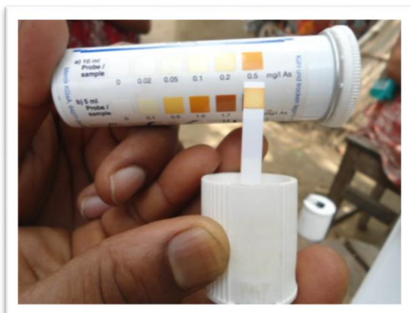
Arsenic testing showing a high level of contamination
