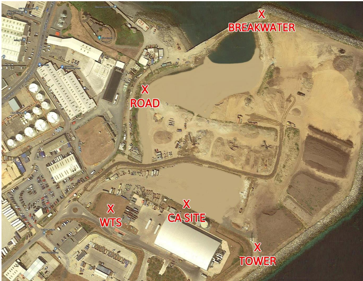
Figure 3. Longue Hougue reclamation site plan showing location and ID of five fixed-position dust flux gauges.
