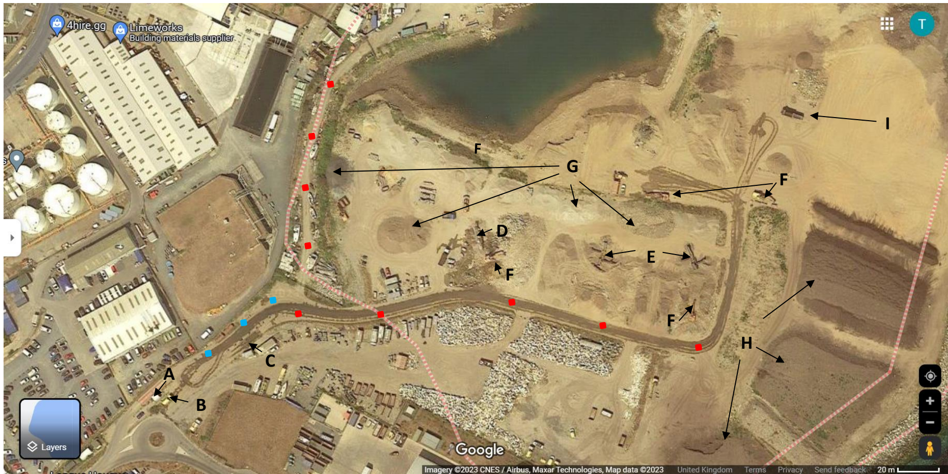
Figure 2. Site layout and key features; A) weighbridge, B) parked water tanker, C) wheel wash (with water tanks opposite), D) crusher, E) mobile screener units, F) tracked excavator, G) aggregate and sand stockpiles, H) compost bunds, and I) mobile compost trommel screen. Note the darker coloured watered roadway and material near the crusher unit. The red blocks indicate trackways where chicanes have been positioned to reduce road going vehicle traffic speed. The blue blocks indicate fixed sprinklers – additional sprinklers for watering stockpiles are not indicated. Actual positioning of plant and stockpiles is subject to change.
